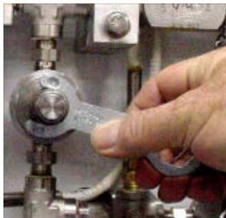
Figure 62. Remove Plunger Assembly
