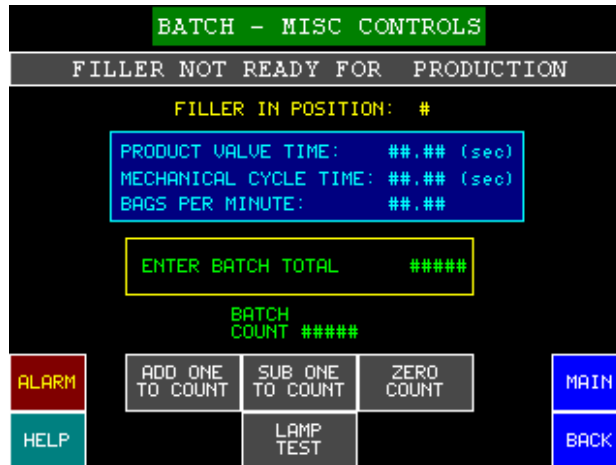
Figure 22. Batch Controls Screen
