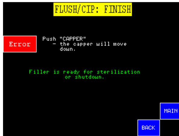
Figure 47. Flush/CIP Finish Screen 2
